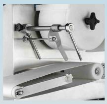
The device is synchronized with the hamburger forming machine work cycle and performs a cleaning stroke every cycle, keeping the wire shiny and clean.
